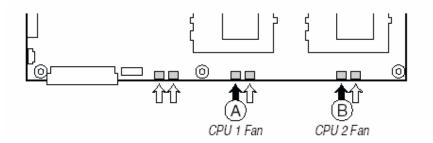
Figure 20: Processor Fan Connectors
